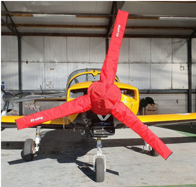
Slingsby T-67 Firefly Insulated Propellor/Spinner Cover
