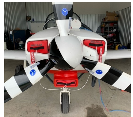
ENGINE PLUGS PREVENT BIRD NEST FOD. Piper Saratoga Engine Cowling Bird's Nest Slingsby T-67 Firefly Engine Inlet Plugs
