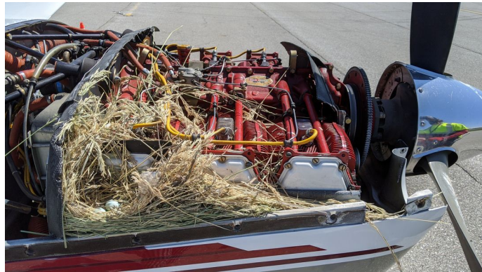
Tecnam P2010 Small Engine Inlet Plug ENGINE PLUGS PREVENT BIRD NEST FOD. Piper Saratoga Engine Cowling Bird's Nest
