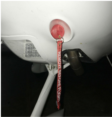
Tecnam P2010 Small Engine Inlet Plug ENGINE PLUGS PREVENT BIRD NEST FOD. Piper Saratoga Engine Cowling Bird's Nest
