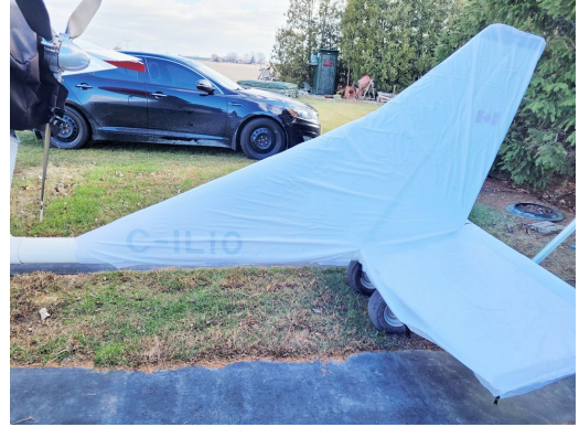
Titan Tornado Empennage Cover, test fit cover
