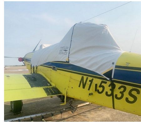
Air Tractor AT-402 Canopy/Hopper Cover
