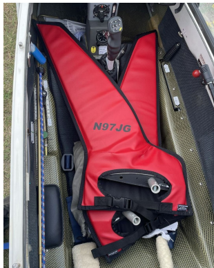
Schempp-Hirth Ventus-2B winglet/wingtip pads
