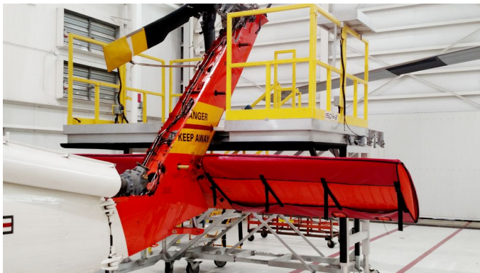
Sikorsky Blackhawk Horizontal Stabilizer Covers, Padded for maintenance protection
