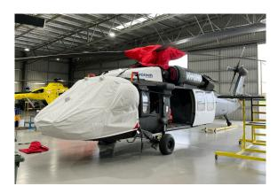
Sikorsky UH-60 Intake/Exhaust Cover Set (IR suppressors) UH 60 Sierra Blackhawk Windshield/Nose Cover, Rotor Mast Cover
