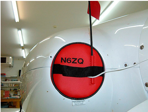
Lancair 320 Engine Inlet Plugs
