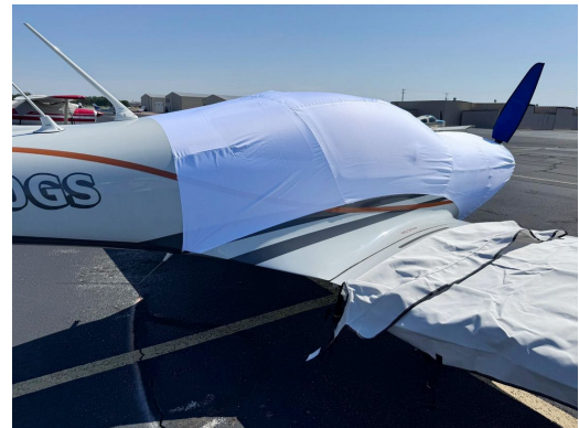
VL3 Canopy/Engine Cover, test fit
