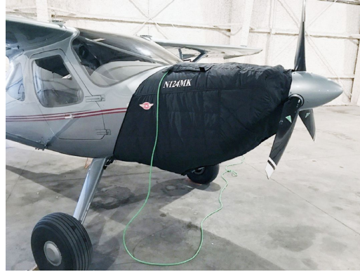
Glasair Aviation Glastar, Sportsman 2+2 Insulated Engine Cover
