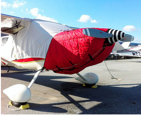
Glastar Insulated Engine Cover
