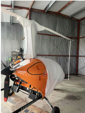
Celier Argon 915 Canopy/Nose Cover, Rotor Mast Cover, test fit covers Celier Argon 915 Rotor Mast Cover, test fit cover
