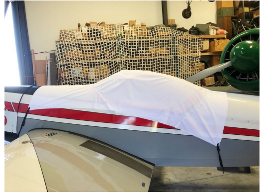
Zlin 526 Canopy Cover, test fit cover
